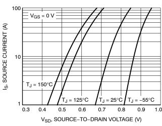
Figure 10. Diode Forward Voltage vs. Current
