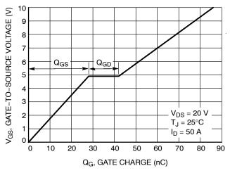
Figure 8. Gate-to-Source Voltage vs. Charge
