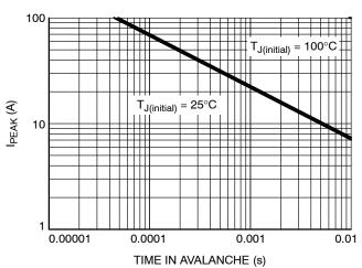
Figure 12. I<sub>PEAK</sub> vs. Time in Avalanche
