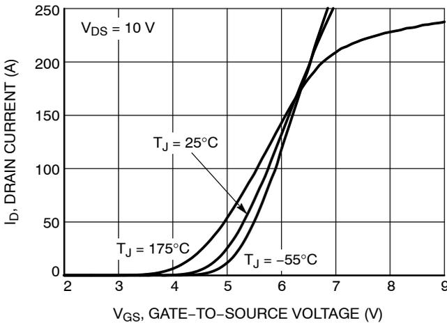
Figure 5. Transfer Characteristics
