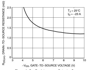
Figure 3. On-Resistance vs. Gate-to-Source Voltage
