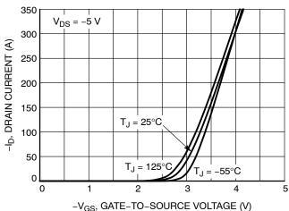
Figure 2. Transfer Characteristics
