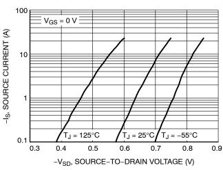
Figure 10. Diode Forward Voltage vs. Current
