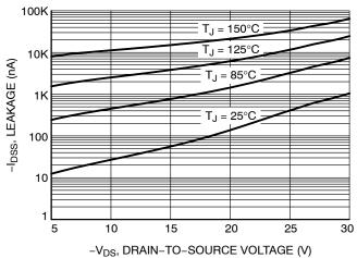
Figure 6. Drain-to-Source Leakage Current vs. Voltage
