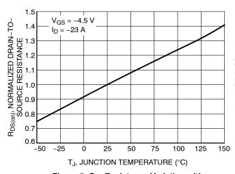
Figure 5. On–Resistance Variation with Temperature
