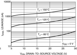
Figure 6. Drain-to-Source Leakage Current vs. Voltage
