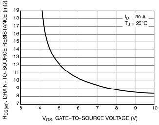
Figure 3. On-Resistance vs. Gate-to-Source Voltage
