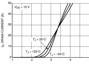
V<sub>GS</sub>, GATE-TO-SOURCE VOLTAGE (V) Figure 2. Transfer Characteristics
