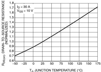
Figure 5. On–Resistance Variation with Temperature
