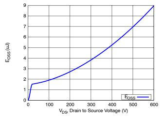
Figure 11. Eoss vs. Drain-to-Source Voltage
