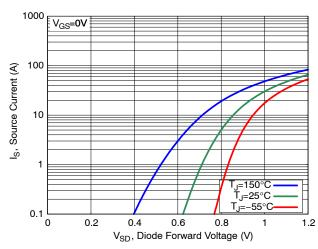
Figure 4. Diode Forward Voltage vs. Source Current
