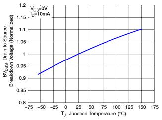
Figure 7. Breakdown Voltage Variation vs. Temperature
