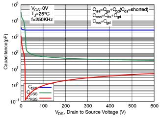
Figure 5. Capacitance Characteristics
