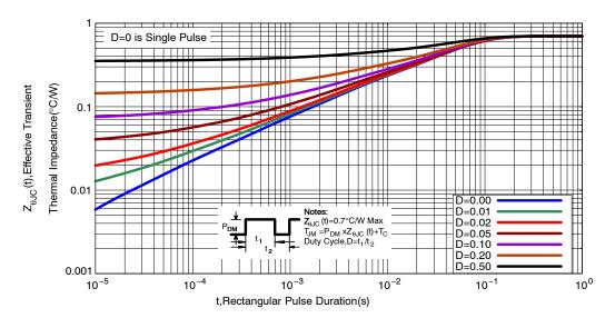
Figure 12. Transient Thermal Impedance
