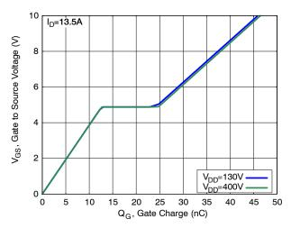
Figure 6. Gate Charge Characteristics
