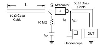
Figure 6. Simplified Schematic of a Typical TLP System
