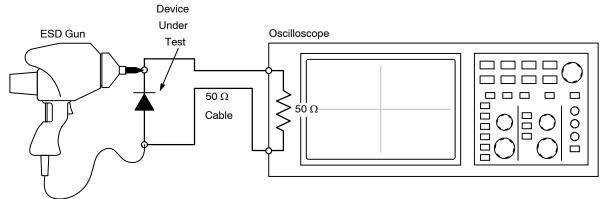
Figure 9. Diagram of ESD Test Setup
