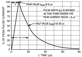
Figure 10. 8 x 20 µs Pulse Waveform
