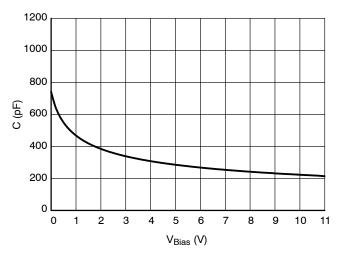
Figure 5. CV Characteristics
