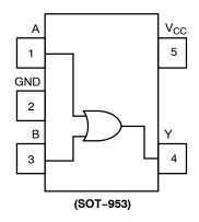
Figure 2. Pinout (Top View)
