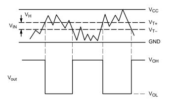
(a) A Schmitt-Trigger Squares Up Inputs With Slow Rise and Fall Times
