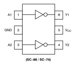
Figure 2. Pinout (Top View)
