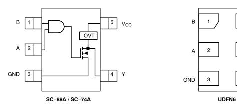
Figure 2. Pinout (Top View)
