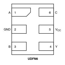
Figure 2. Pinout (Top View)
