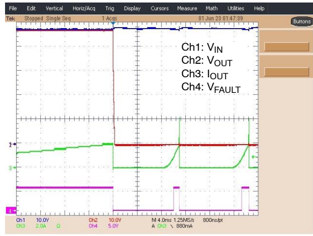
Figure 19. I_{TH} Overcurrent Event on Auto-retry Device
