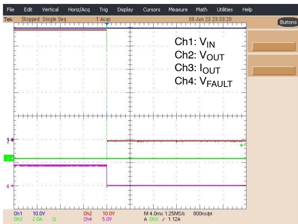
Figure 22. Short Circuit Event on Latching Device
