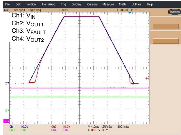
Figure 15. Turning on a Single Output with the Input Voltage While Another Output is On (EN pin pull-up or floated)
