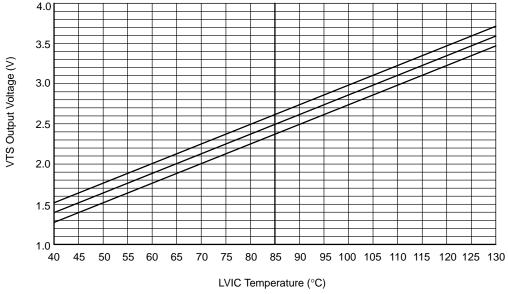
Figure 4. Temperature of LVIC versus VOT Characteristics
