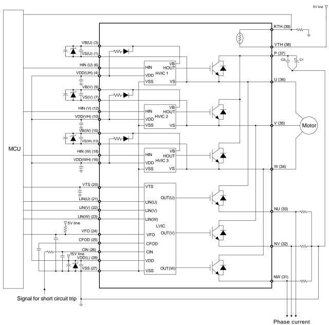
Figure 2. Application Schematic - Adjustable Option
