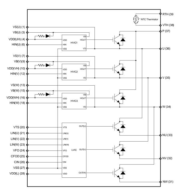
Figure 3. Equivalent Block Diagram
