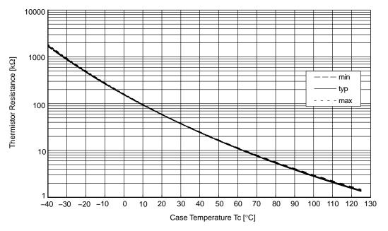
Figure 5. Thermistor Resistance versus Case Temperature
