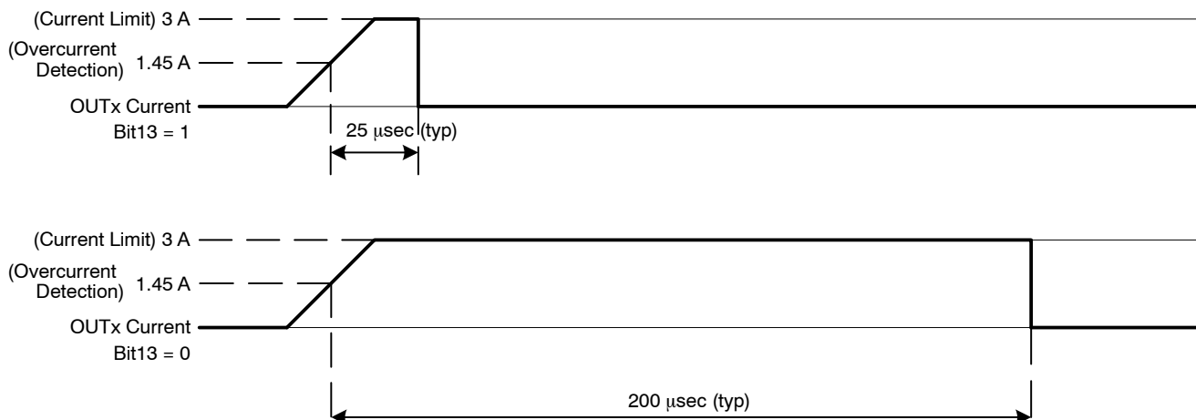
Figure 13. Output Current Shutdown Control
