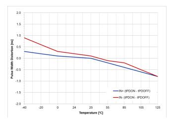
Figure 48. Pulse Width Distortion vs. Temperature (CLOAD = 0 nF)
