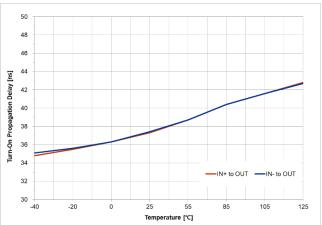
Figure 45. Turn-on Propagation Delay vs. Temperature (C<sub>LOAD</sub> = 0 nF)
