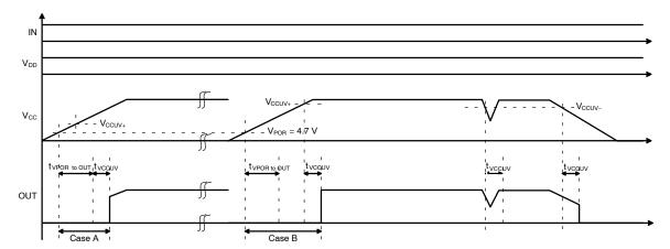
Figure 53. V<sub>CC</sub> Power-up UVLO Delay Time
