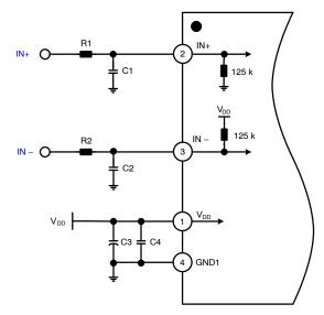
Figure 57. Schematic of Input Stage
