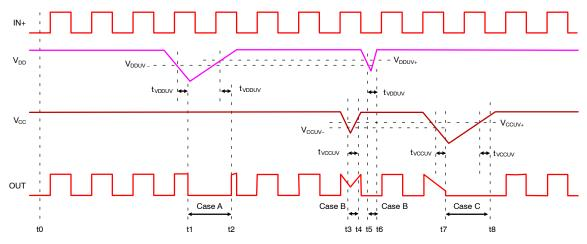
Figure 52. Timing Chart Under-Voltage Lockout Protection
