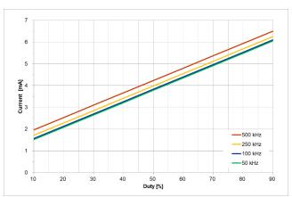
Figure 14.  $V_{DD}$  Operating Current vs. Duty ( $V_{DD} = 5 \text{ V}$ , IN+ Switching with Different Frequency, IN- = 0 V)
