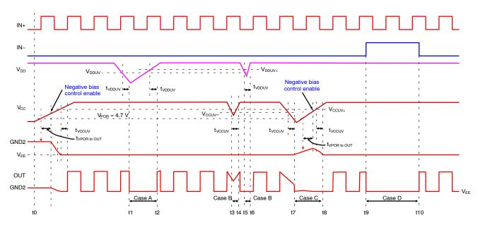
Figure 51. Overall Operating Waveforms Definitions
