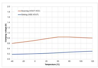
Figure 42. Clamping Voltage vs. Temperature
