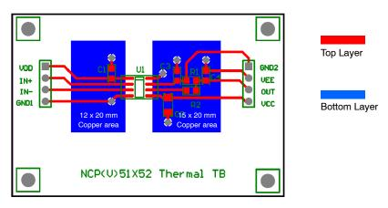
Figure 5. Reference Layout for the Type-B
