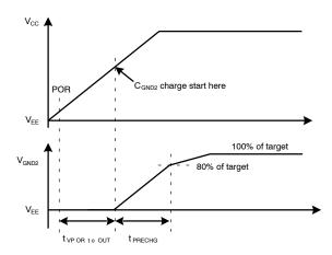
Figure 56. Timing Chart Negative Bias Control During Precharge
