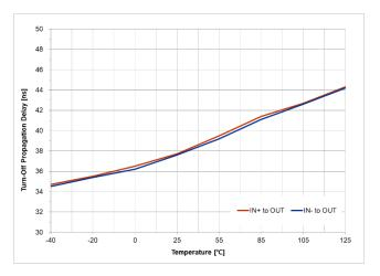
Figure 46. Turn-off Propagation Delay vs. Temperature (C<sub>LOAD</sub> = 0 nF)
