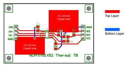
Figure 4. Reference Layout for the Type-A
