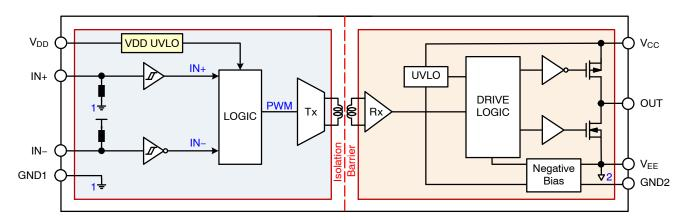
Figure 2. Simplified Block Diagram
