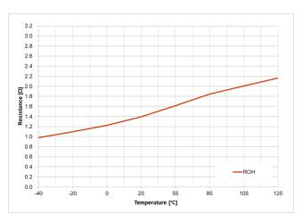
Figure 43. Output Resistance at High State vs. Temperature
