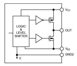
Figure 58. Schematic of Output Stage
