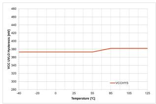
Figure 24.  $V_{CC}$  6-V UVLO Threshold vs. Temperature
