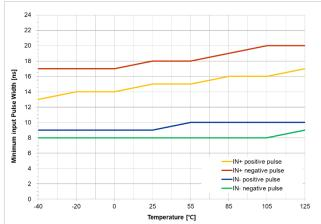
Figure 49. Minimum Input Pulse Width vs. Temperature
