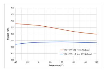
Figure 16. Quiescent V<sub>CC</sub> Supply Current vs. Temperature
