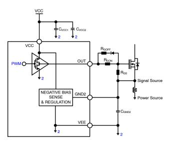
Figure 54. Supplying V<sub>EE</sub> with Negative Bias Control
