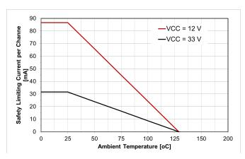
Figure 6. Thermal Derating Curve for Safety–related Limiting Current ( $\theta_{JA} = 100^{\circ}$ C/W) (Note 7)
