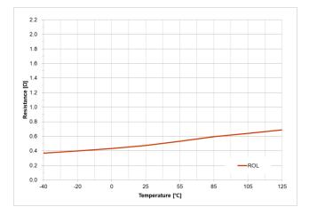
Figure 44. Output Resistance at Low State vs. Temperature
