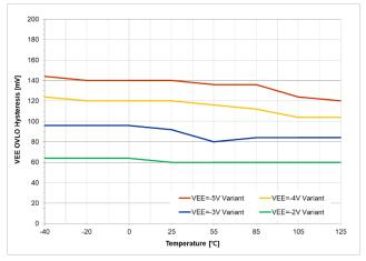
Figure 38. V<sub>EE</sub> Bias Over Voltage Threshold vs. Temperature
