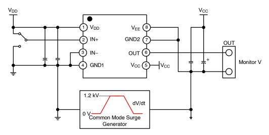
Figure 59. Common Mode Transient Immunity Test Circuit
