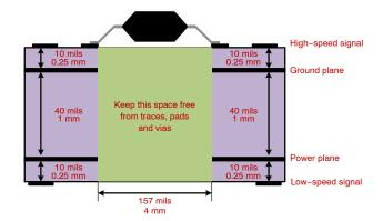
Figure 60. Recommended Layer Stack
