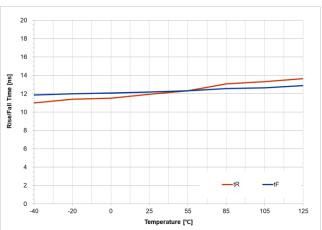
Figure 47. Rise/Fall Time vs. Temperature  $(C_{LOAD} = 1.8 \text{ nF})$
