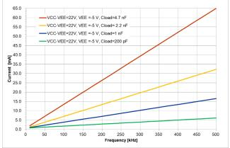
Figure 21. V<sub>CC</sub> Operating Current vs. Switching Frequency (V<sub>CC</sub> – V<sub>EE</sub> = 22 V, V<sub>EE</sub> = -5 V and Different C<sub>LOAD</sub>)
