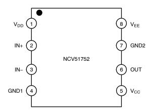
Figure 3. Pin Connections – SOIC-8 NB (Top View)
