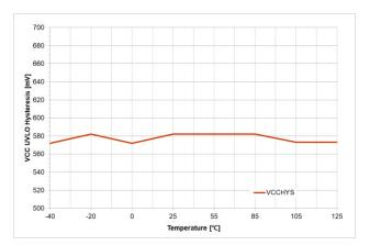
Figure 26. V<sub>CC</sub> 8–V UVLO Threshold vs. Temperature
