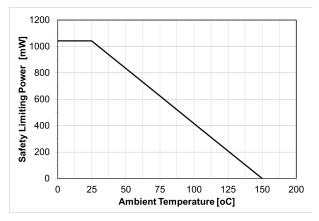
Figure 9. Thermal Derating Curve for Safety–related Limiting Power ( $\theta_{JA}$  = 120°C/W) (Note 8)
