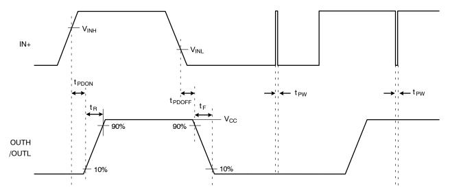
Figure 50. Switching Time Definition
