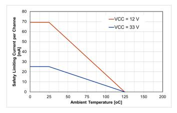
Figure 8. Thermal Derating Curve for Safety–related Limiting Current ( $\theta_{JA}$  = 120°C/W) (Note 8)
