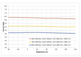
Figure 17. V<sub>CC</sub> Operating Current vs. Temperature
