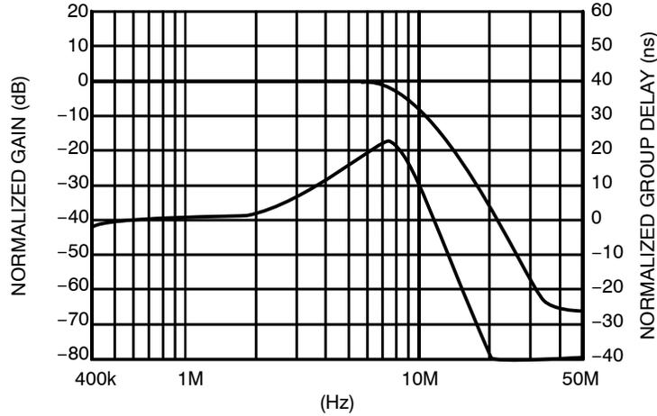
**Figure 18. SD Frequency Response and Group Delay**
