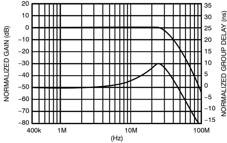
**Figure 19. HD Frequency Response and Group Delay**
