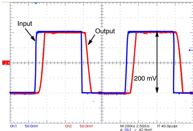
Figure 13. SD Small Signal Response
