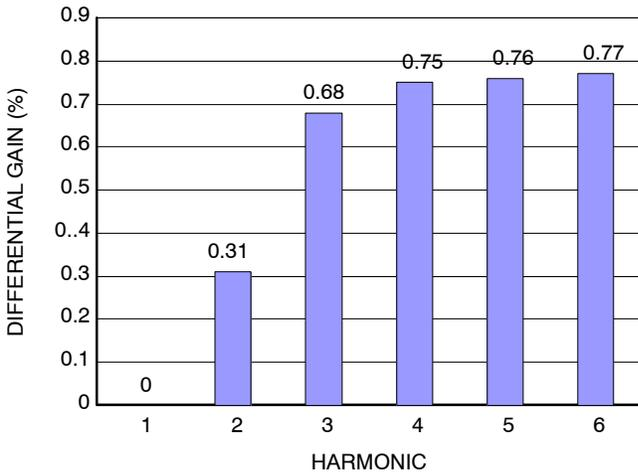
**Figure 20. SD Differential Gain**
