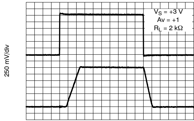
Figure 24. 3 V Non-Inverting Large Signal Pulse Response
