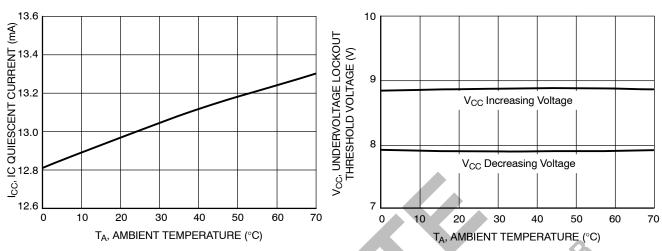
Figure 5. IC Quiescent Current vs. Ambient **Temperature**
