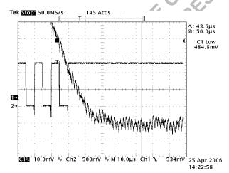
Figure 14. Dynamic VID Settling Time Falling
