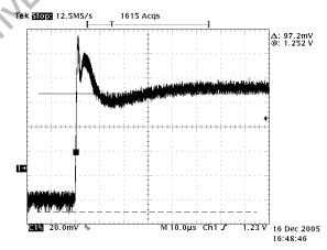
Figure 11. Typical Load Release Event
