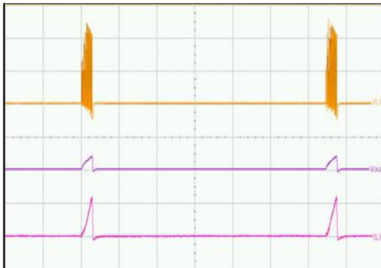
(VIN = 5 V, VOUT = 1.8 V, IOU T = Current Limit, no CSS) Upper Trace: LX Pin Voltage, 5 V / div Middle Trace: Output Voltage, 2 V / div Lower Trace: Inductor Current, 2 A / div Time = 500 μs / div
