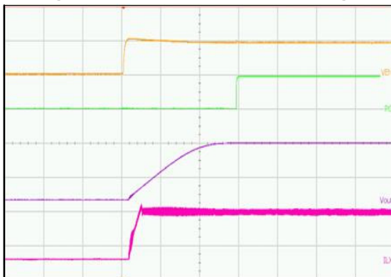
(VIN = 5 V, VOUT = 1.8 V, IOU T = 3 A, CSS = 4.7 nF) Upper Trace: Enable Pin Voltage, 5 V / div Second Trace: Power Good Pin Voltage, 5 V / div Third Trace: Output Voltage, 2 V / div Lower Trace: Inductor Current, 2 A / div Time = 2 ms / div
