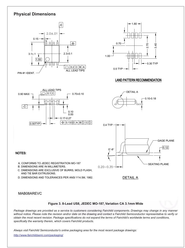
NC7NP14 — TinyLogic<sup>®</sup> ULP Triple Inverter with Schmitt Trigger Input
