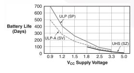
TinyLogic ULP and ULP-A with up to 50% less power consumption can extend your battery life significantly.
