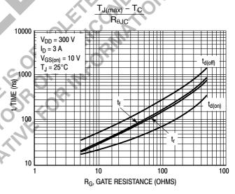
Figure 9. Resistive Switching Time Variation versus Gate Resistance
