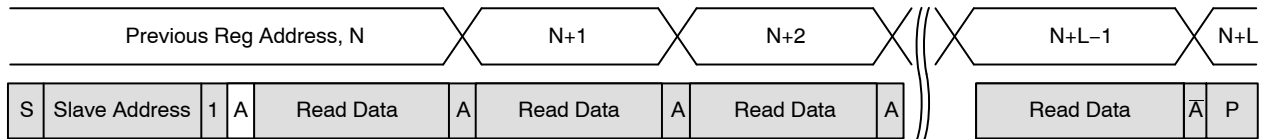
Figure 19. Sequential READ, Start from Current Location
