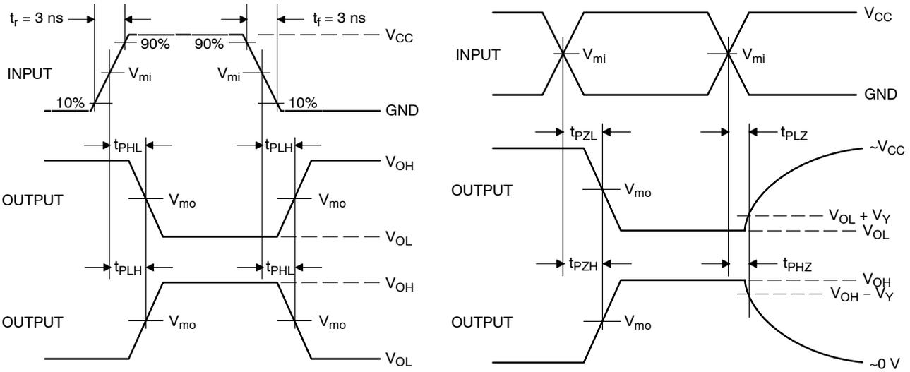
**Figure 4. Switching Waveforms**
