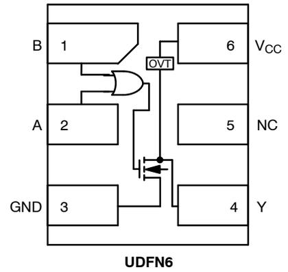
Figure 2. Pinout (Top View)
