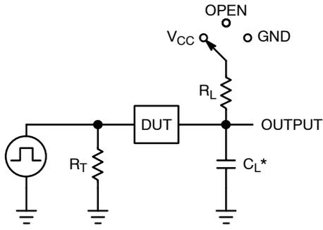
$C_L$  includes probe and jig capacitance
