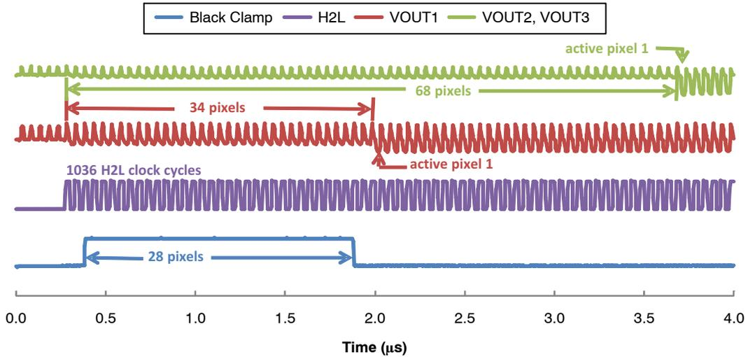
Figure 32. Video Output at Each Line Start
