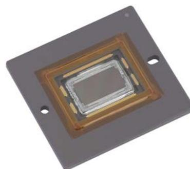
**Figure 1. KAE-02150 Interline CCD
