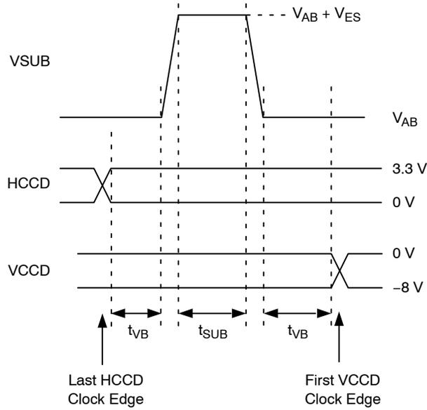
**WARNING:** Do not clock the EMCCD register while the electronic shutter pulse is high.
