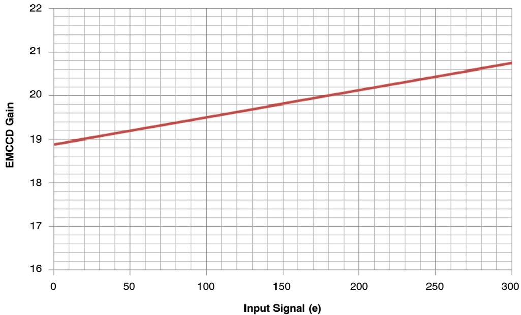
NOTE: The EMCCD voltage was set to provide 20x gain with an input of 180 electrons.
