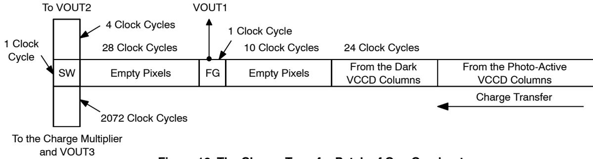
Figure 16. The Charge Transfer Patch of One Quadrant
