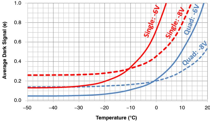
NOTE: Both are for a HCCD frequency of 20 MHz. The VCCD low level voltage is shown for each curve.
