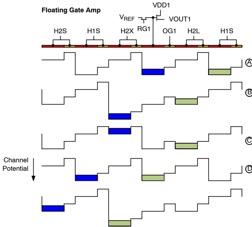
NOTE: The blue and green rectangles represent two separate charge packets. The direction of charge transfer is from right to left.
