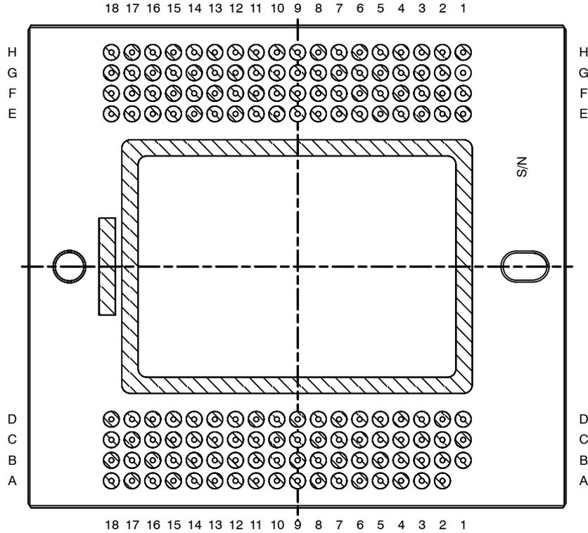
Figure 5. PGA with TEC Pin Descriptions – Bottom View
