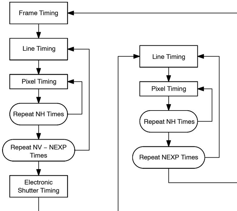
**Figure 40. The Image Readout Timing Flow Chart**
