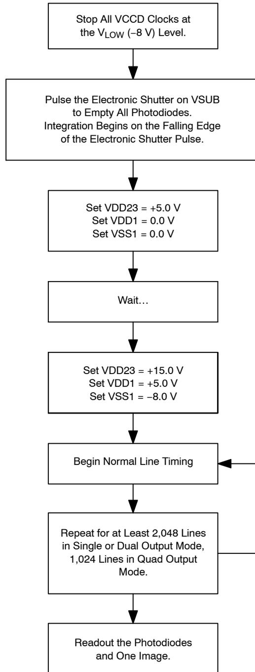
Figure 41. Timing Flow Chart for Long Integration Time
