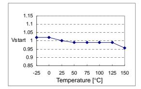
Figure 6. Start Threshold Voltage
