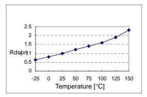
Figure 14. Static Drain-Source on Resistance
