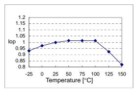
Figure 3. Operating Supply Current
