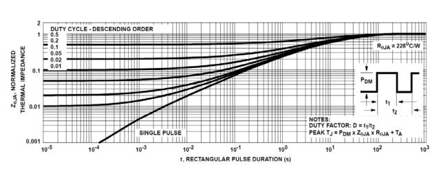
Figure 3. NORMALIZED MAXIMUM TRANSIENT THERMAL IMPEDANCE
