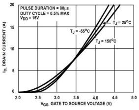
Figure 7. TRANSFER CHARACTERISTICS
