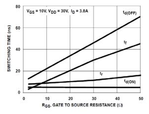
Figure 16. SWITCHING TIME vs GATE RESISTANCE
