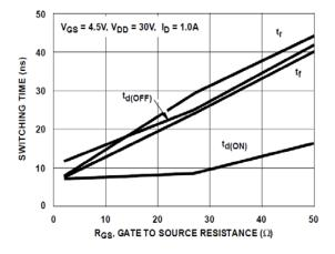
Figure 15. SWITCHING TIME vs GATE RESISTANCE
