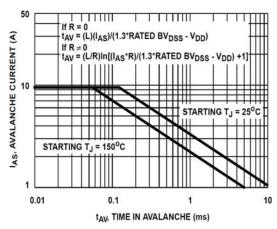
Figure 6. UNCLAMPED INDUCTIVE SWITCHING CAPABILITY
