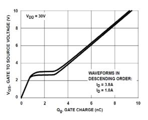
Figure 14. GATE CHARGE WAVEFORMS FOR CONSTANT GATE CURRENT
