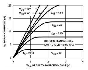
Figure 8. SATURATION CHARACTERISTICS
