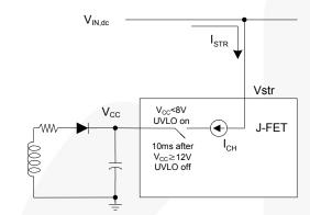
Figure 13. Startup Circuit
