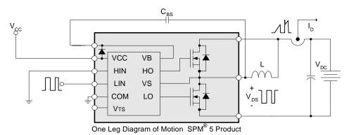
Figure 8. Switching and RBSOA (Single-pulse) Test Circuit (Low-side)
