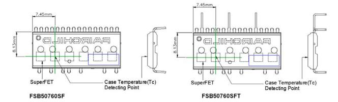
Figure 5. Case Temperature Measurement
