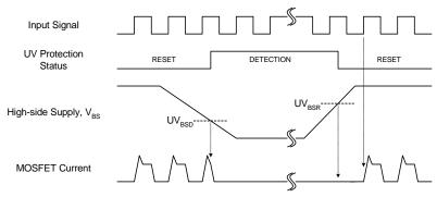
Figure 10. Under-Voltage Protection (High-Side)
