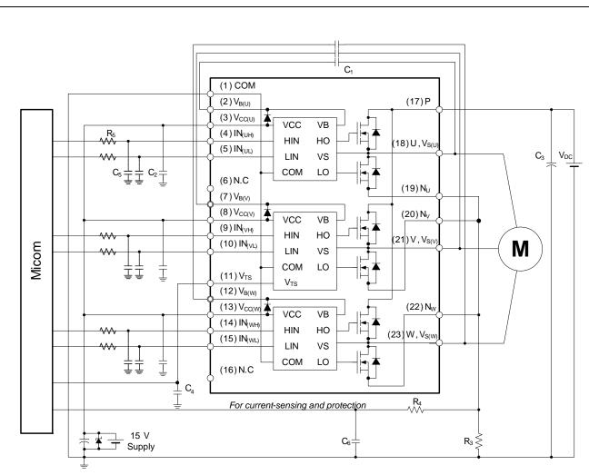
Figure 11. Example of Application Circuit
