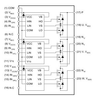
Figure 2. Pin Configuration and Internal Block Diagram (Bottom View)
