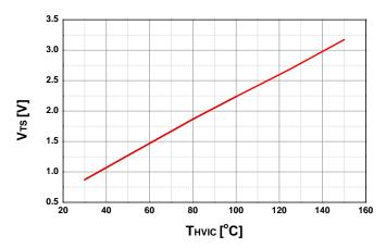
Figure 6. Temperature Profile of V⊤s (Typical)
