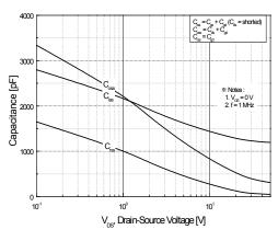
Figure 5. Capacitance Characteristics
