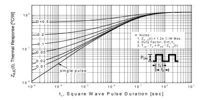
Figure 11. Transient Thermal Response Curve
