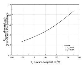
Figure 8. On-Resistance Variation vs. Temperature
