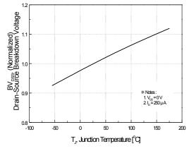
Figure 7. Breakdown Voltage Variation vs. Temperature
