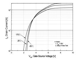
Figure 2. Transfer Characteristics
