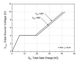
Figure 6. Gate Charge Characteristics
