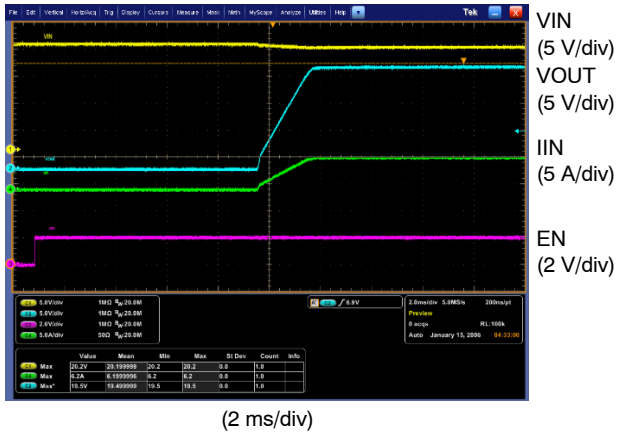
Figure 12. VIN = 20 V, ROUT = 3.4 Ω
