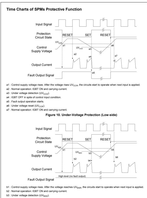
b4 : IGBT OFF in spite of control input condition, but there is no fault output signal.
