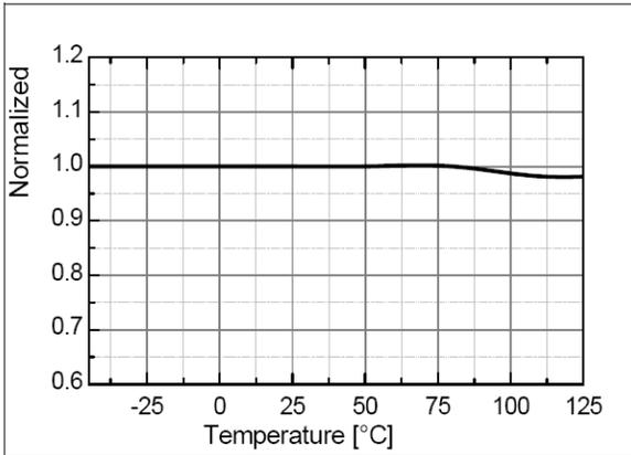
Figure 16. Output Voltage High (V<sub>OH</sub>) vs. T<sub>A</sub>
