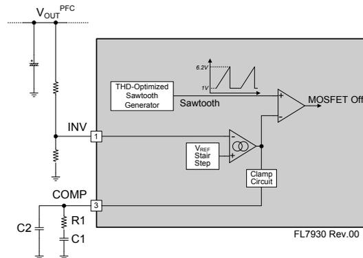
**Figure 32. Control Circuit**
