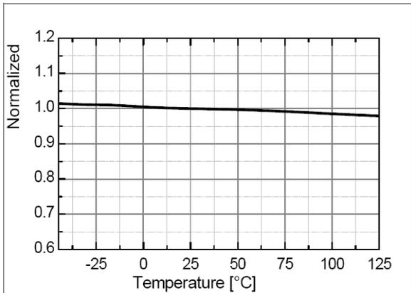
**Figure 9. Output Upper Clamp Voltage (V<sub>EAH</sub>) vs. T<sub>A</sub>**
