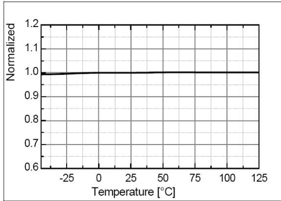
**Figure 5. Start Threshold Voltage (V<sub>START</sub>) vs. T<sub>A</sub>**
