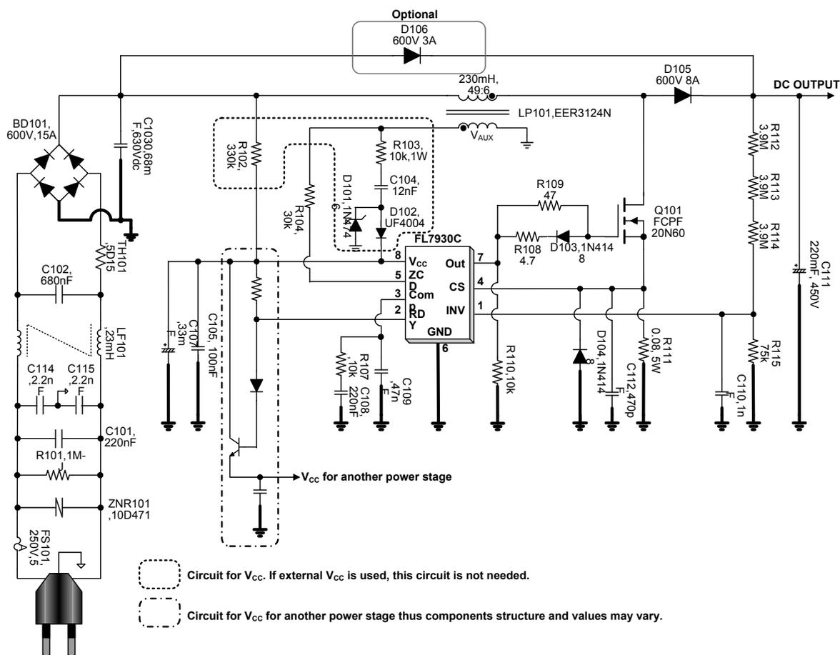
Figure 45. Demonstration Circuit
