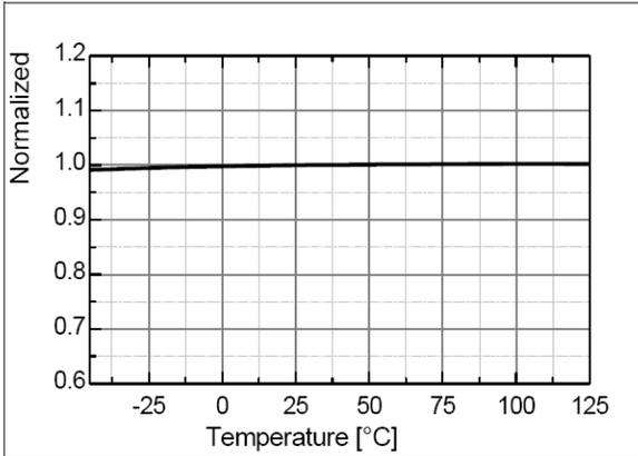
**Figure 4. Voltage Feedback Input Threshold 1 (V<sub>REF1</sub>) vs. T<sub>A</sub>**
