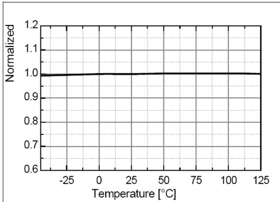
Figure 19. Output Ready Voltage (V<sub>RDY</sub>) vs. T<sub>A</sub>
