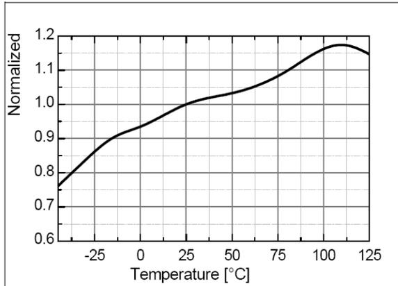
Figure 17. Output Voltage Low (V<sub>OL</sub>) vs. T<sub>A</sub>
