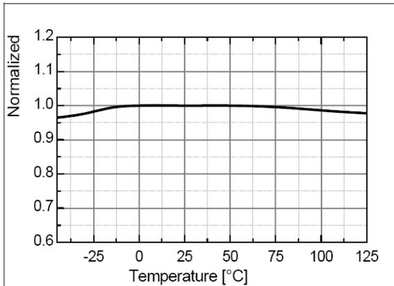
**Figure 8. Operating Supply Current (I<sub>OP</sub>) vs. T<sub>A</sub>**
