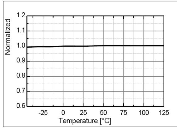
Figure 21. OVP Threshold Voltage (V<sub>OVP</sub>) vs. T<sub>A</sub>
