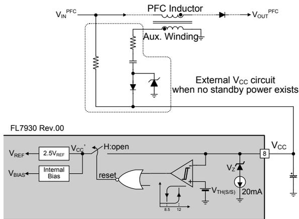
Figure 22. Startup Circuit
