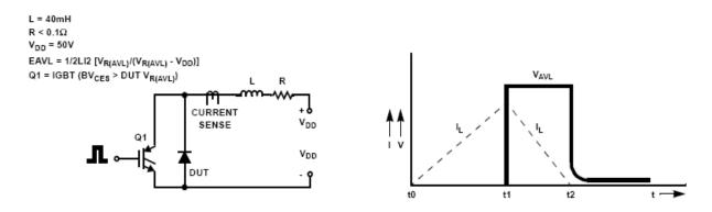
Figure 2. Unclamped Inductive Switching Test Circuit & Waveform
