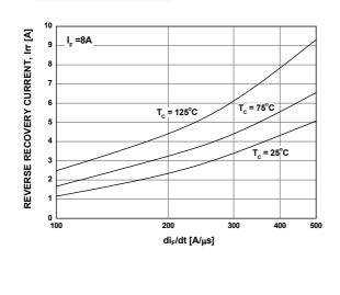
Figure 4. Typical Reverse Current
