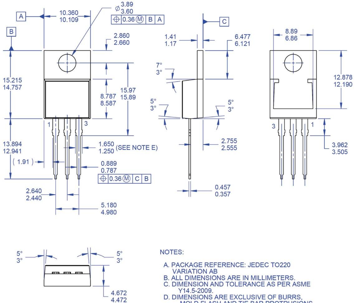
**Figure 19. TO-220, Molded, 3-Lead, Jedec Variation AB**
