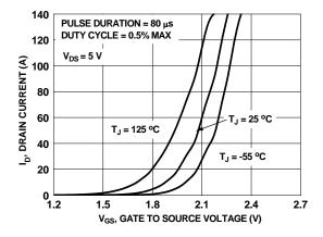
Figure 5. Transfer Characteristics
