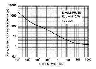
Figure 12. Single Pulse Maximum Power Dissipation
