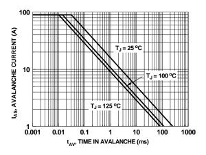
Figure 9. Unclamped Inductive Switching Capability
