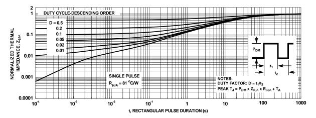
Figure 13. Junction-to-Ambient Transient Thermal Response Curve
