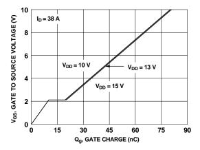
Figure 7. Gate Charge Characteristics
