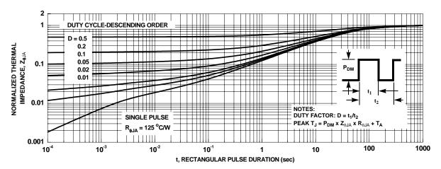
Figure 13. Junction-to-Ambient Transient Thermal Response Curve
