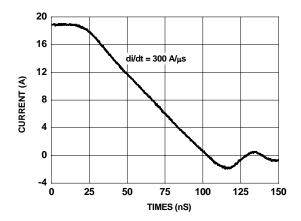
Figure 14. Body Diode Reverse Recovery Characteristics
