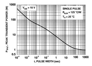
Figure 12. Single Pulse Maximum Power Dissipation
