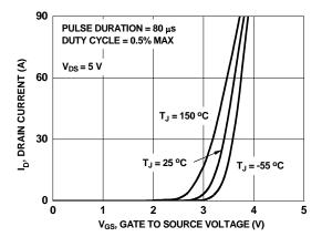
Figure 5. Transfer Characteristics
