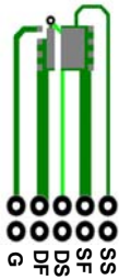
c. 125\text{ }^\circ\text{C}/\text{W} when mounted on a minimum pad of 2 oz copper
