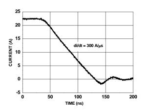
Figure 13. FDMC2514SDC SyncFET body diode reverse recovery characteristic
