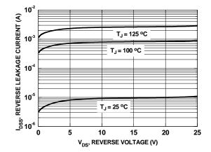
Figure 14. SyncFET body diode reverse leakage versus drain-source voltage
