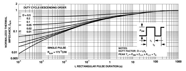
Figure 11. Junction-to-Ambient Transient Thermal Response Curve
