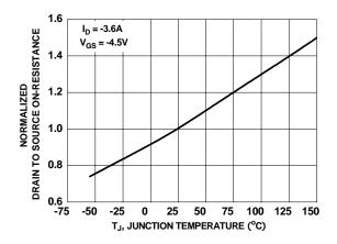
Figure 3. Normalized On-Resistance vs Junction Temperature
