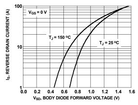
Figure 7. Forward Diode Characteristics
