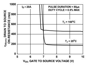
Figure 10. Rdson vs Gate Voltage
