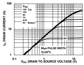
Figure 8. Saturation Characteristics
