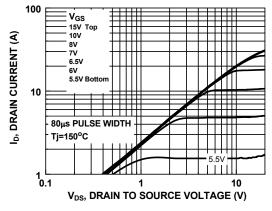
Figure 9. Saturation Characteristics
