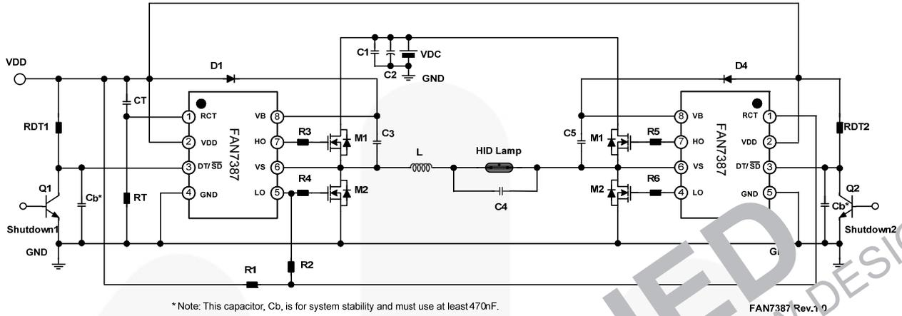
Figure 3. Typical Application Circuit for Full-Bridge Converter
