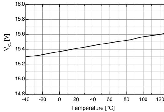
Figure 17. V<sub>CL</sub> vs. Temperature
