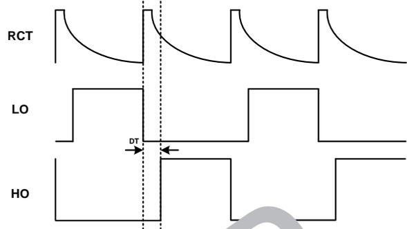
Figure 8. Basic Operating Waveforms of Self-Oscillation Method
