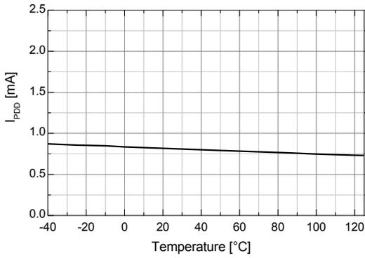
Figure 18. I<sub>PDD</sub> vs. Temperature
