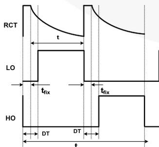
Figure 31. Typical Waveforms of RCT, LO and HO
