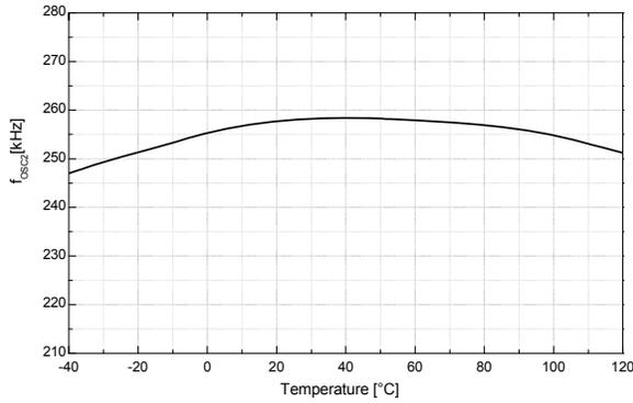
Figure 24. Operating Frequency 2 vs. Temperature
