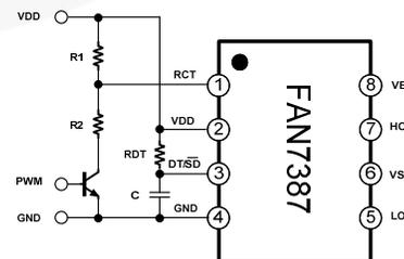
Figure 34. Gate Driver Using External PWM Signal
