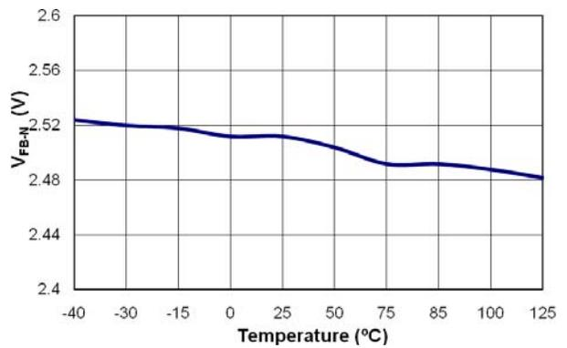
**Figure 11. FB Threshold Voltage for Frequency Reduction (V<sub>FB-N</sub>) vs. Temperature**
