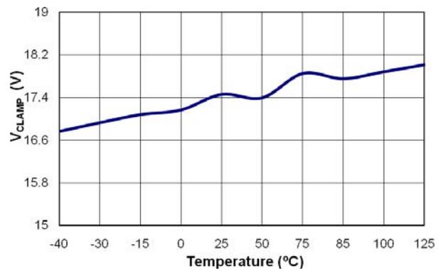
**Figure 17. GATE Output Clamping Voltage ( $V_{CLAMP}$ ) vs. Temperature**
