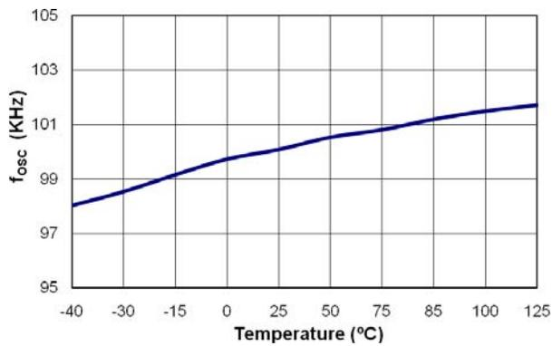
**Figure 10. Center Frequency (f<sub>OSC</sub>) vs. Temperature**
