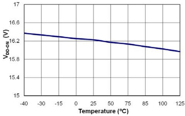
**Figure 6. Turn-On Threshold Voltage (V<sub>DD-ON</sub>) vs. Temperature**
