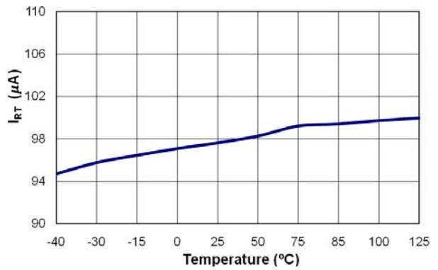
**Figure 21. Output Current of RT Pin (I<sub>RT</sub>) vs. Temperature**
