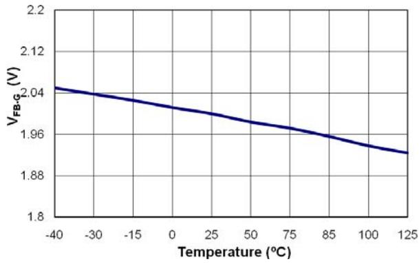
**Figure 12. FB Voltage at  $f_{OSC-G}$  ( $V_{FB-G}$ ) vs. Temperature**
