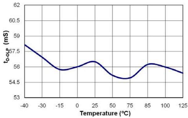
**Figure 14. Open-Loop Protection Delay ( $t_{D-OLP}$ ) vs. Temperature**
