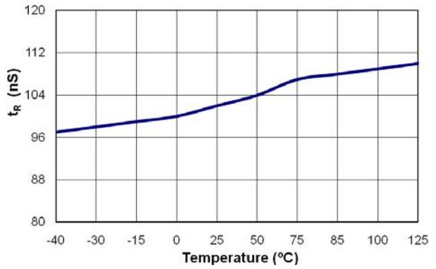
**Figure 19. Rising Time (t<sub>R</sub>) vs. Temperature**
