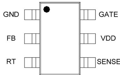
Figure 4. Pin Assignments
