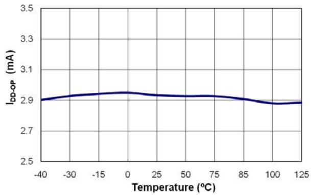
**Figure 8. Operating Current (I<sub>DD-OP</sub>) vs. Temperature**
