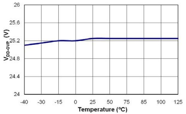
**Figure 9. V<sub>DD</sub> Over-Voltage Protection (V<sub>DD-OVP</sub>) vs. Temperature**
