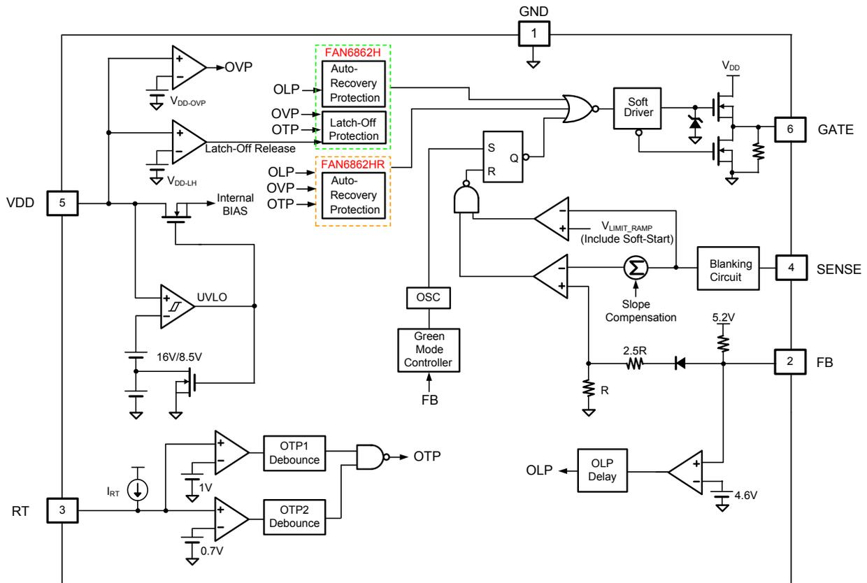
Figure 2. Block Diagram
