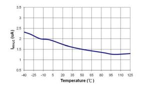
Figure 14. HV Pin Leakage Current After Startup (I<sub>HV-LC</sub>) vs. Temperature
