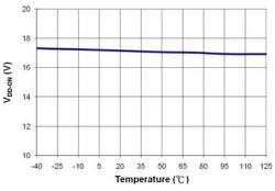
Figure 11. Start Threshold Voltage (V<sub>DD-ON</sub>) vs. Temperature
