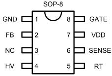
Figure 4. Pin Configuration (Top View)
