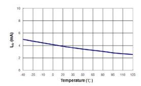
Figure 13. Supply Current Drawn from HV Pin (I<sub>HV</sub>) vs. Temperature
