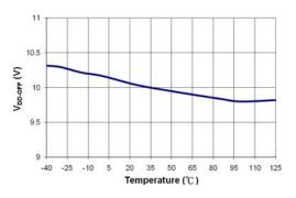
Figure 12. Minimum Operating Voltage (V<sub>DD-OFF</sub>) vs. Temperature
