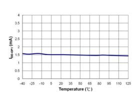
Figure 10. Operation Supply Current (I<sub>DD-OP1</sub>) vs. Temperature
