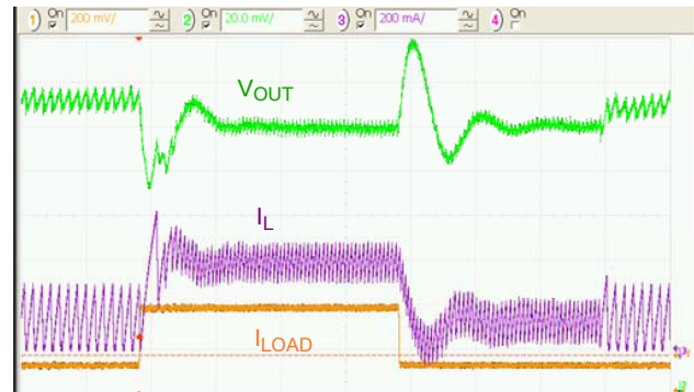
Figure 22. Load Transient 150 mA to 400 mA, V_{IN} = 3.6\text{ V} , t_{RISE} = t_{FALL} = 100\text{ ns} , 5 \mu\text{s}/\text{div} .
