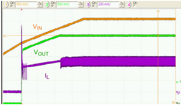
Figure 17. Startup Ramping V_{IN} = V_{EN} with 500 mA Load, 1 ms/div.
