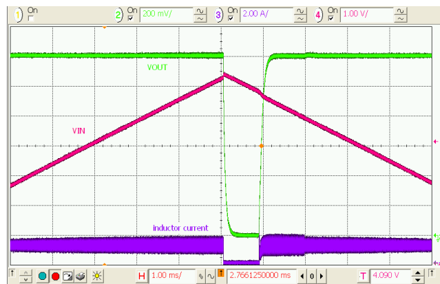
Figure 29. Input Over-Voltage Protection
