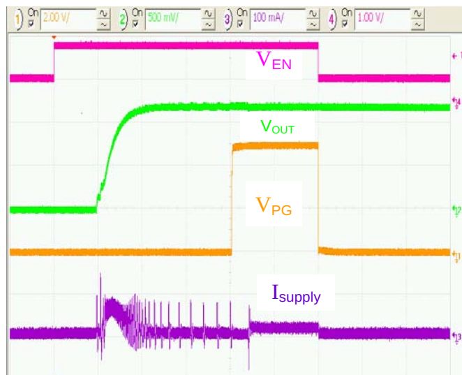
Figure 15. Soft-Start: EN Voltage Raised After V_{IN} = 5.0\text{ V} , I_{LOAD} = 0 , Horizontal Scale = 100\text{ }\mu\text{s/div} .
