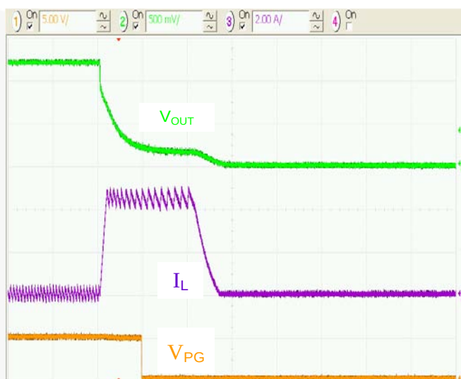
Figure 20. V_{OUT} to GND Short Circuit, 5 \mu\text{s}/\text{div} .
