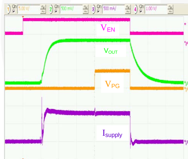
Figure 17. Soft-Start: EN Pin Raised after V_{IN} = 5.0\text{ V} , R_{LOAD} = 400\text{ m}\Omega , C_{OUT} = 100\text{ }\mu\text{F} , Horizontal Scale = 100\text{ }\mu\text{s/div} .
