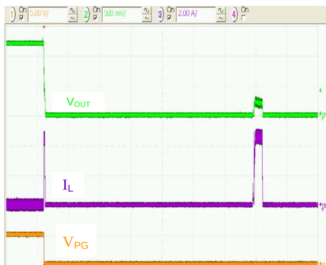
Figure 19. V_{OUT} to GND Short Circuit, 200 \mu\text{s}/\text{div} .
