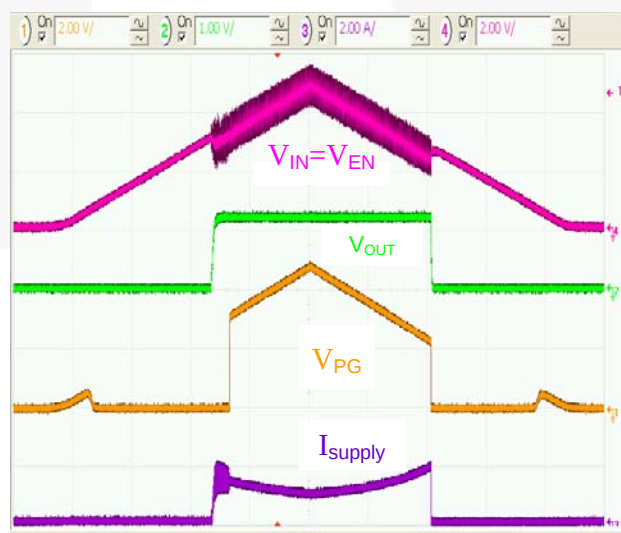
Figure 18. Soft-Start: EN Pin Tied to VCC, R_{LOAD} = 400\text{ m}\Omega , C_{OUT} = 100\text{ }\mu\text{F} , Horizontal Scale = 1\text{ ms/div} .
