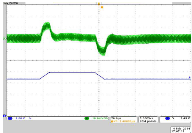
Figure 14. Line Transient, 200 mA Load, 10 µs Step
