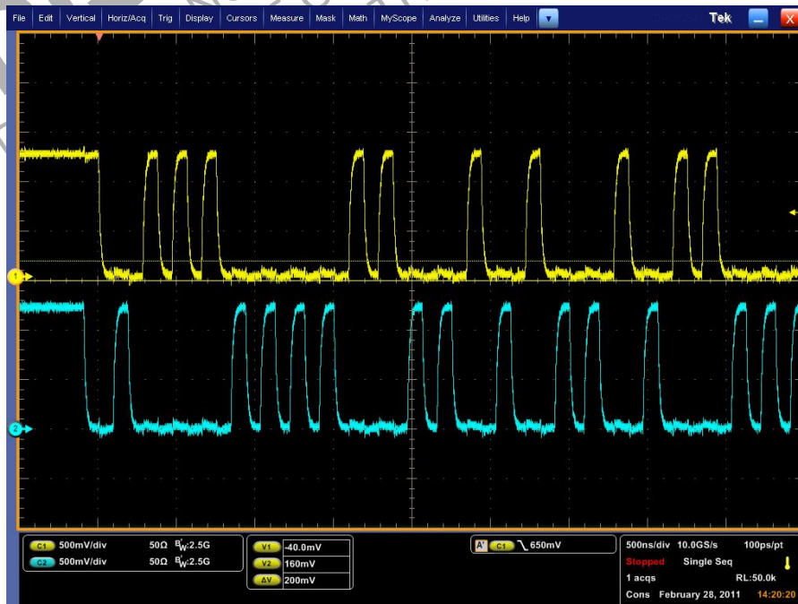
Figure 5. EMI4192 MIPI D-PHY LP Mode Measured Results
