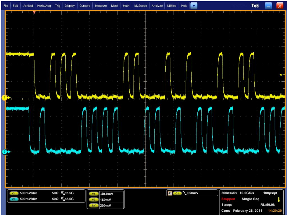
Figure 8. EMI4183MU MIPI D-PHY LP Mode Measured Results
